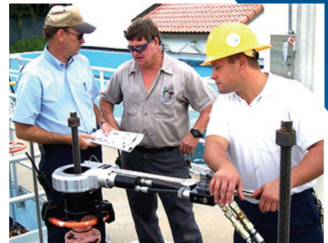
Hydraulic drive RS-2 single user operation
